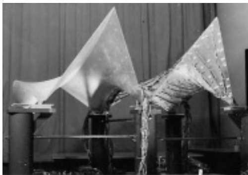
Fig. 8.2-3: Example of an object with unknown directions of principal stresses (from [8-2]) - a plastic model of a concrete-shell roof for investigation by stress analysis using strain gages
